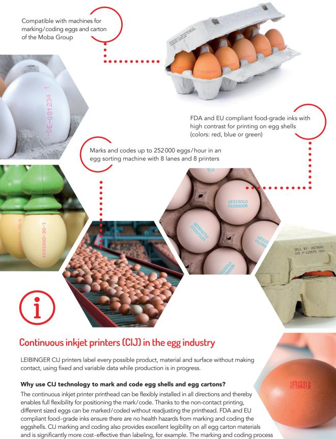
is greatly simplified thanks to the complete plug-and-play integration in egg sorting machines. That makes CIJ technology the only complete economical solution for marking and coding eggs and egg cartons.
