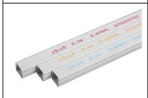
Examples of marking imprints on extrusion products.
