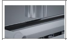
The LEIBINGER IQJET marks cables during the extrusion process.
